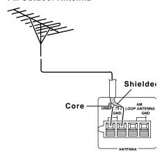
**Note:** Grounding is not necessary for reception, but we recommend it to avoid damage from lightning when you use an outdoor FM antenna and for better FM reception. Use a separate piece of thick polyvinyl insulated wire to connect the **GND** terminal to an earth ground such as a metal cold-water pipe.
